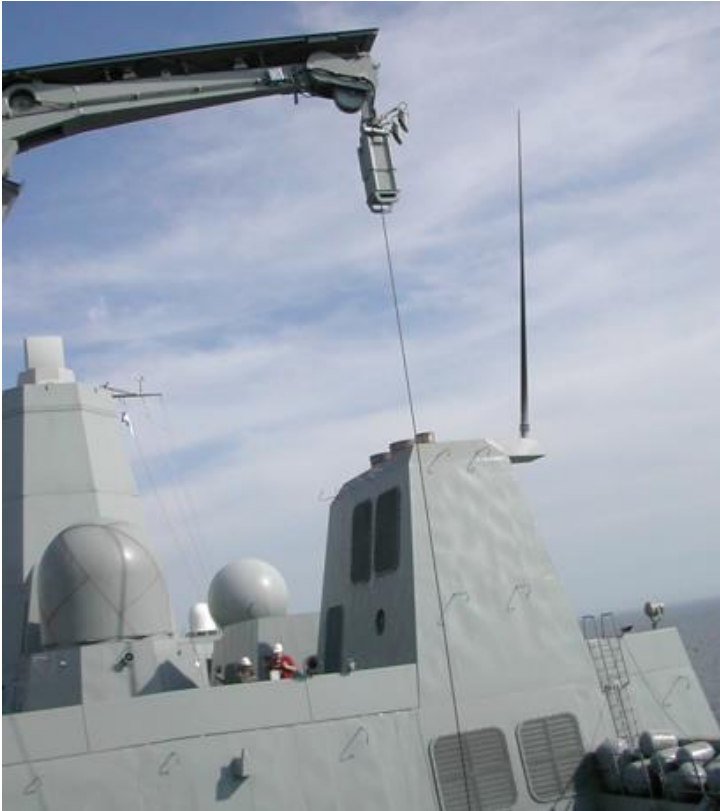
HF whip & crane cable
