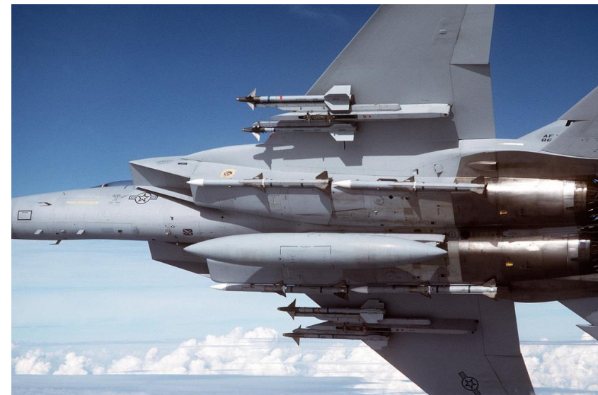
Figure 2: Captive carriage of numerous EO on an aircraft [2]
