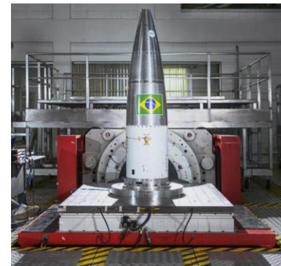
Figure 6: Horizontal single shaker test setup [6]
