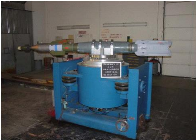
Figure 1: Single shaker single axis test setup [8]
