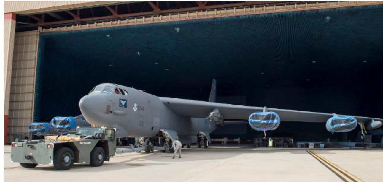
B-52 Bomber being prepped for HERO testing at Benefield Anechoic Facility, Edwards AFB
